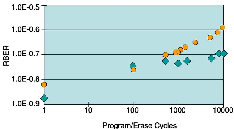
Picture 4: Examples of increasing RBER with frequent program/erase cycles
