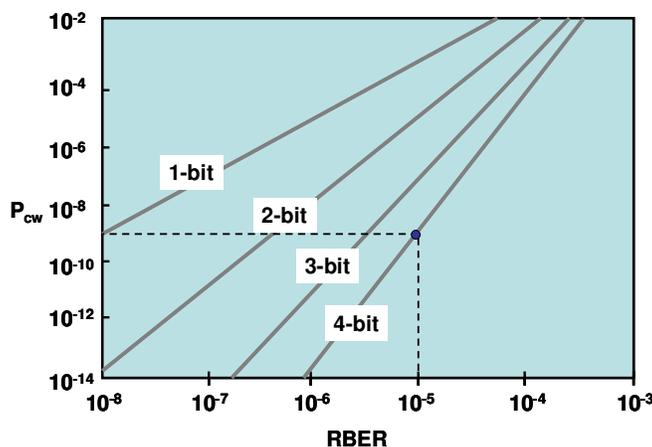
**Picture 3: Controller ECC improves bit error rate**
