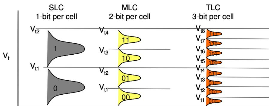
Picture 2: Voltage Levels for SLC, MLC and TLC flash technologies
